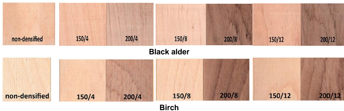
Fig. 5. Colour changes of veneers before and after densification at 150°C and 200°C and pressure levels of 4, 8 and 12 MPa [28]
