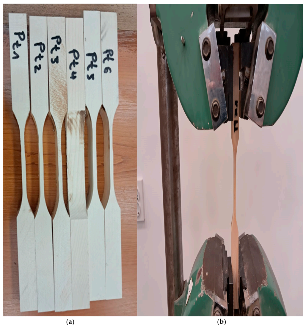
Figure 2. Determination of the tensile strength parallel to the wood fibers: (a) sample shape; (b) fixing between the blades of the tensile testing machine.
