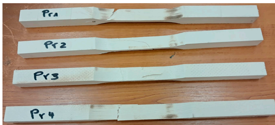
Figure 10. Shape of the breaks parallel to the wood fibers.
