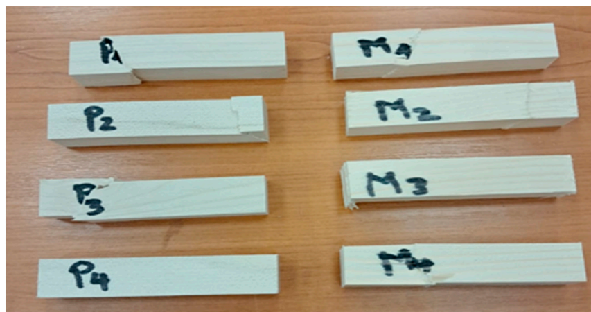
Figure 8. Fracture patterns of wood in compressive strength tests parallel to the wood fibers.
