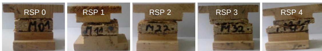
Fig. 9. Rupture zones of the samples during IB test
