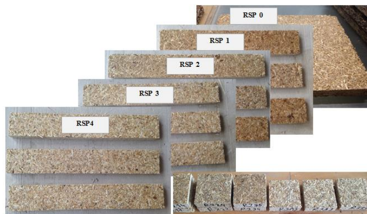
Fig. 2. Samples cut for testing the mechanical and physical properties of the experimental panels
