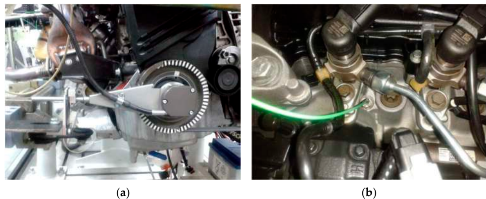
Figure 3. The sensors used for determining the variation of the cylinder pressure depending on the crank angle: (a) Crankshaft angle encoder; (b) Cylinder pressure sensor.
