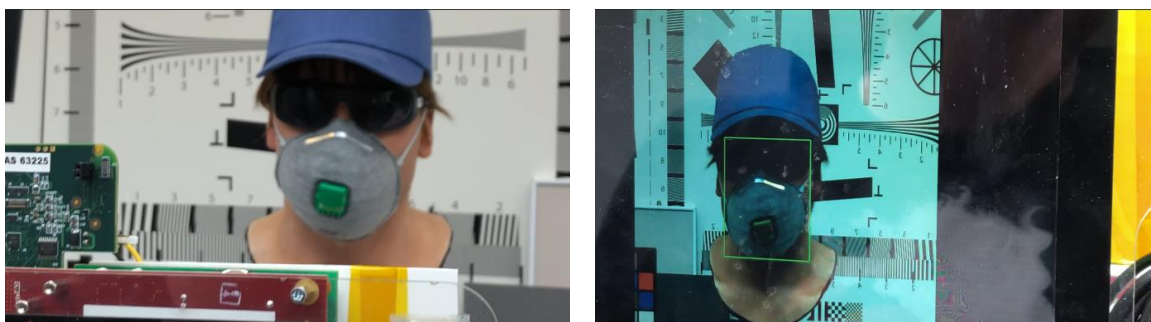
Figure A2. RT operation of the FPGA-based "PoC"—the masked subject and the camera system board (left); the result of detection (right).
