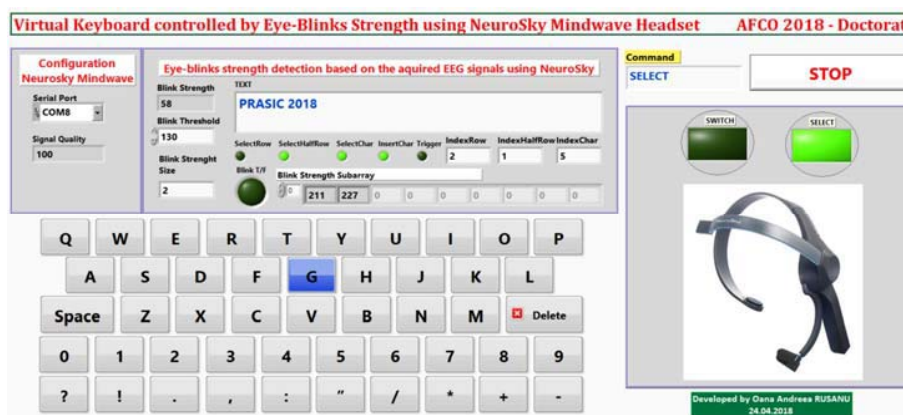
Figure 1. Front Panel (user-interface) of the LabVIEW based virtual keyboard controlled by eye-blinks strength via EEG signal acquired using NeuroSky Mindwave headset.
