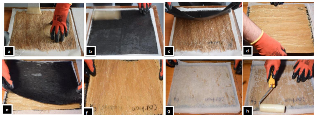
Figure 3. Experimental composite panel manufacturing; (a). resin applied by hand lay-up technique on the face layer; (b). carbon twill layer; (c). placement of carbon twill layer as the 2nd layer; (d). the 3rd layer of date palm fibers arranged transversally to the direction of faces; (e). the carbon twill 4-th layer; (f). the face layer oriented longitudinally; (g). silicon paper sheet for protection; (h). pre-pressing the laminate.
