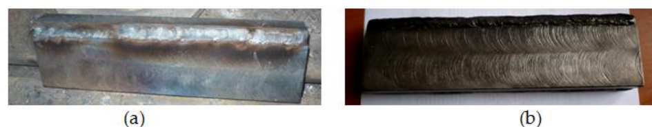
Figure 8. Deposit aspect: (a) rot bead; (b) surface bead.
