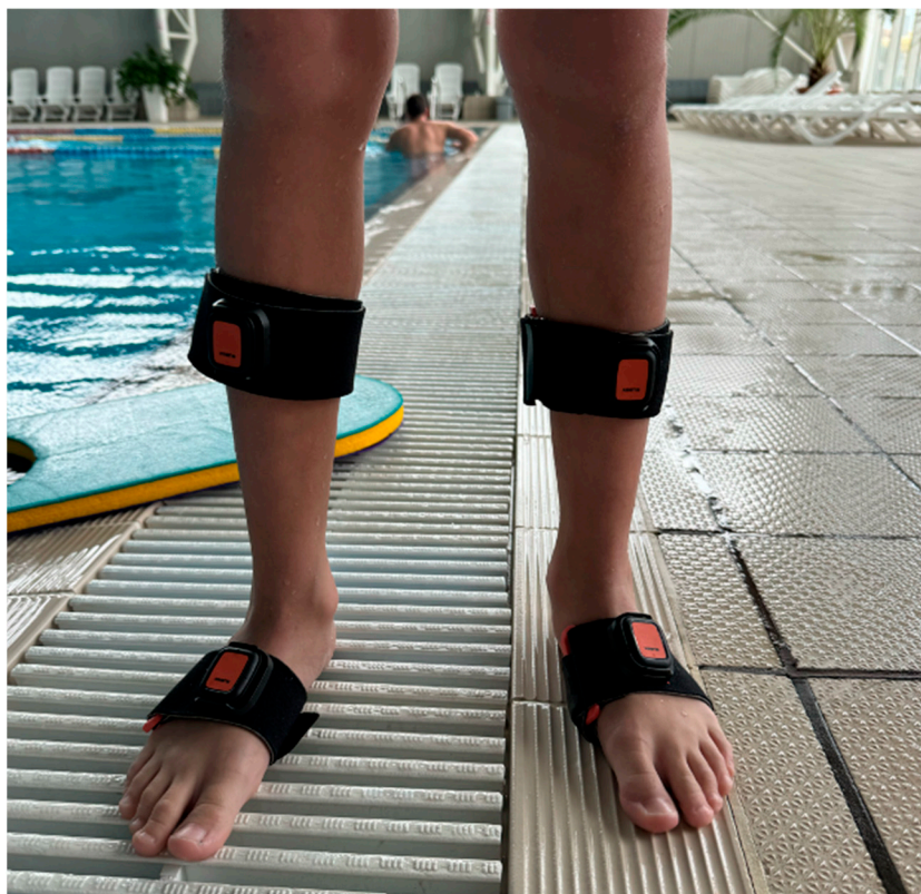
Figure 1. Placement of wearable inertial sensors on the lower limbs. Sensors were attached bilaterally to the shanks and feet to capture segment-level kinematics relevant to breaststroke kick mechanics.
