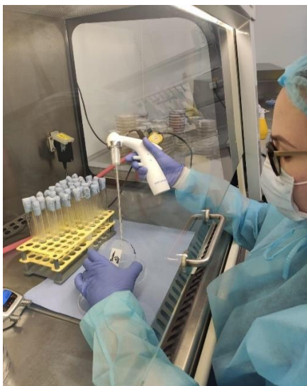
Fig. 8. Transfer the dilution to the Petri dish Source: the authors – 2021
