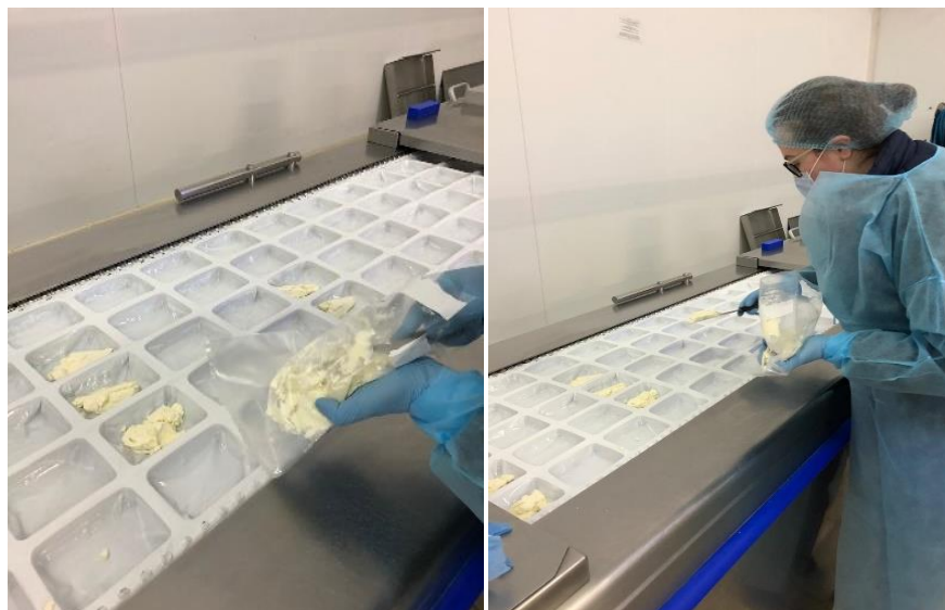
Fig. 4. Placing the cheese (telemea) in the shapes of the packaging machine
