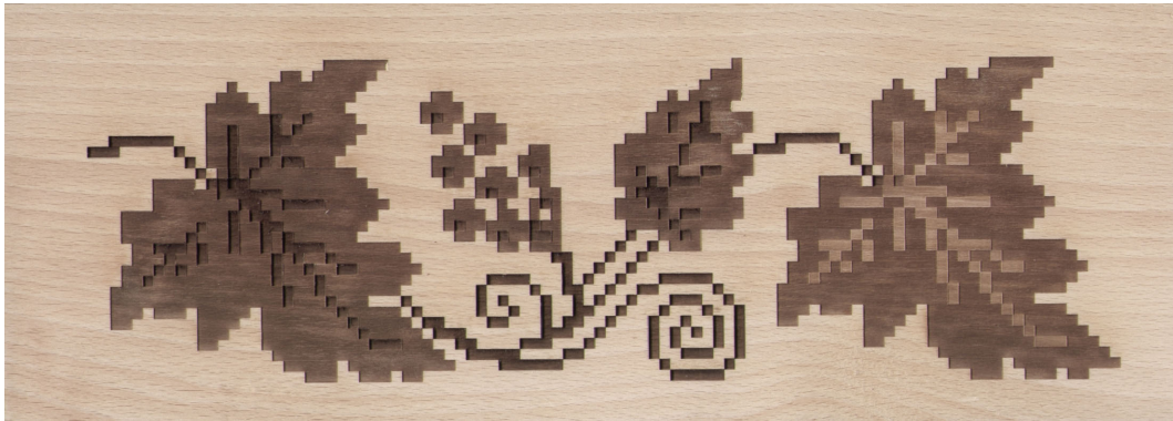
Figure 6. Laser engraved model using 20% of maximum power of the equipment for yellow (laser output of 30 W), 30% of maximum power of the equipment for red (laser output of 45 W), and 70% of maximum power of the equipment for black (laser output of 105 W).
