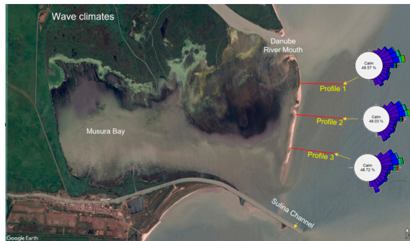
Figure 9. The locations of the coastal profiles (red lines) and the associated wave climates represented as wave roses. Satellite image from Google Earth Pro, dated 11 July 2017.
