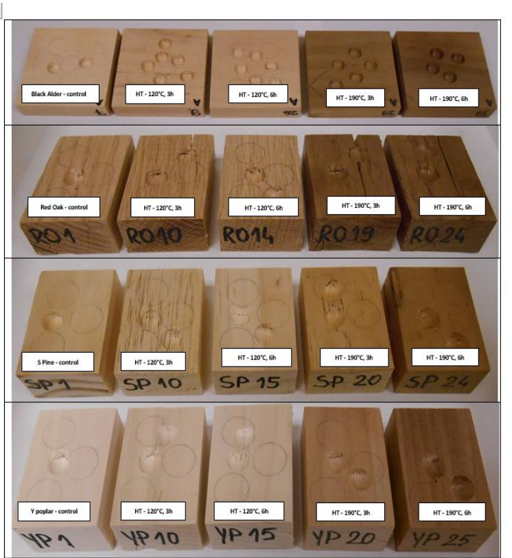
Fig. 8. Discoloration of control and heat-treated samples [18]
