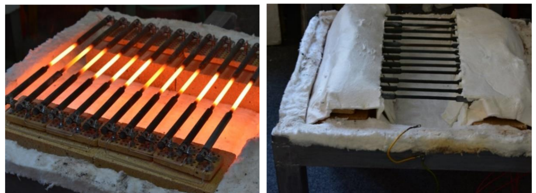
Figure 4. Silite bars/rods during operation, and their thermal insulation.
