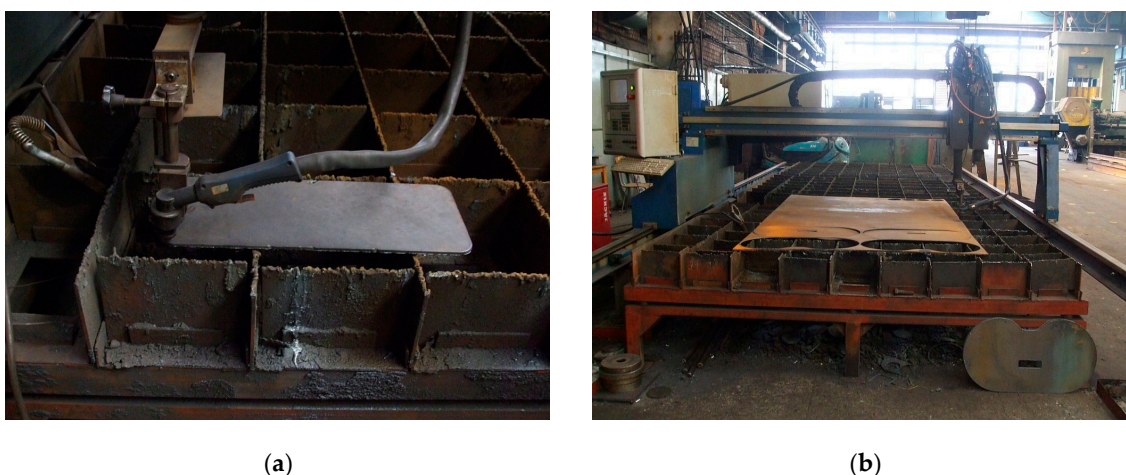
Figure 4. ComCut 31 CNC cutting machine equipped with (a) plasma cutting torch; (b) oxy-fuel torch.
