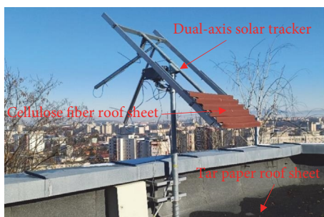
FIGURE 8: Test setup for the inclined positioning of the PV test bed on top of the fiberboard.
