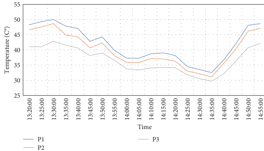
FIGURE 31: Back surface temperatures vs. time for the latitude-tilted PV test bed with some panels covered in dust on October 30, 2023.
