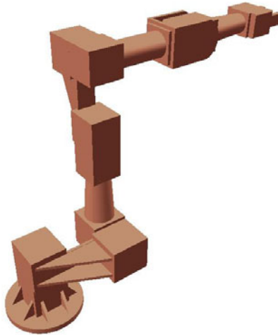
Fig. 1. PowerCube arm exported from CATIA in C++/OGRE
