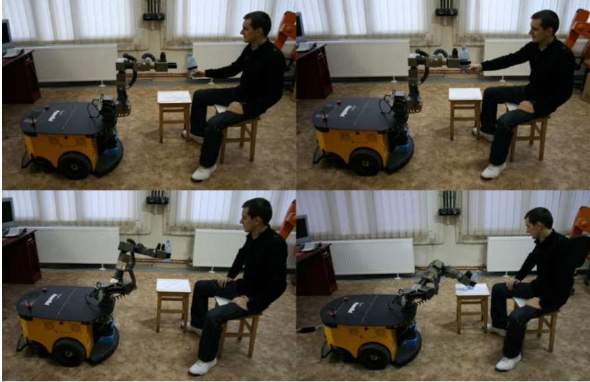
Fig. 6. Real environment scenario; the robot receives from subject a plastic bottle, which will be placed on a chair
