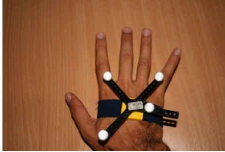
Fig. 4. Passive optical markers mounted on subject's hand
