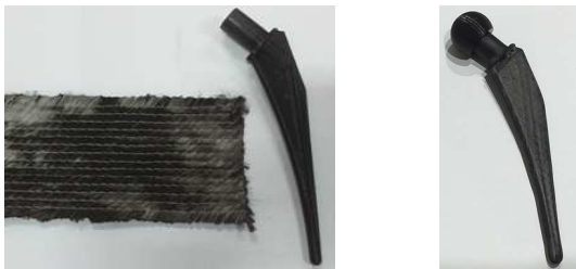
Fig. 2. Coating the core in the carbon fiber sleeve with epoxy resin [4], [11]
