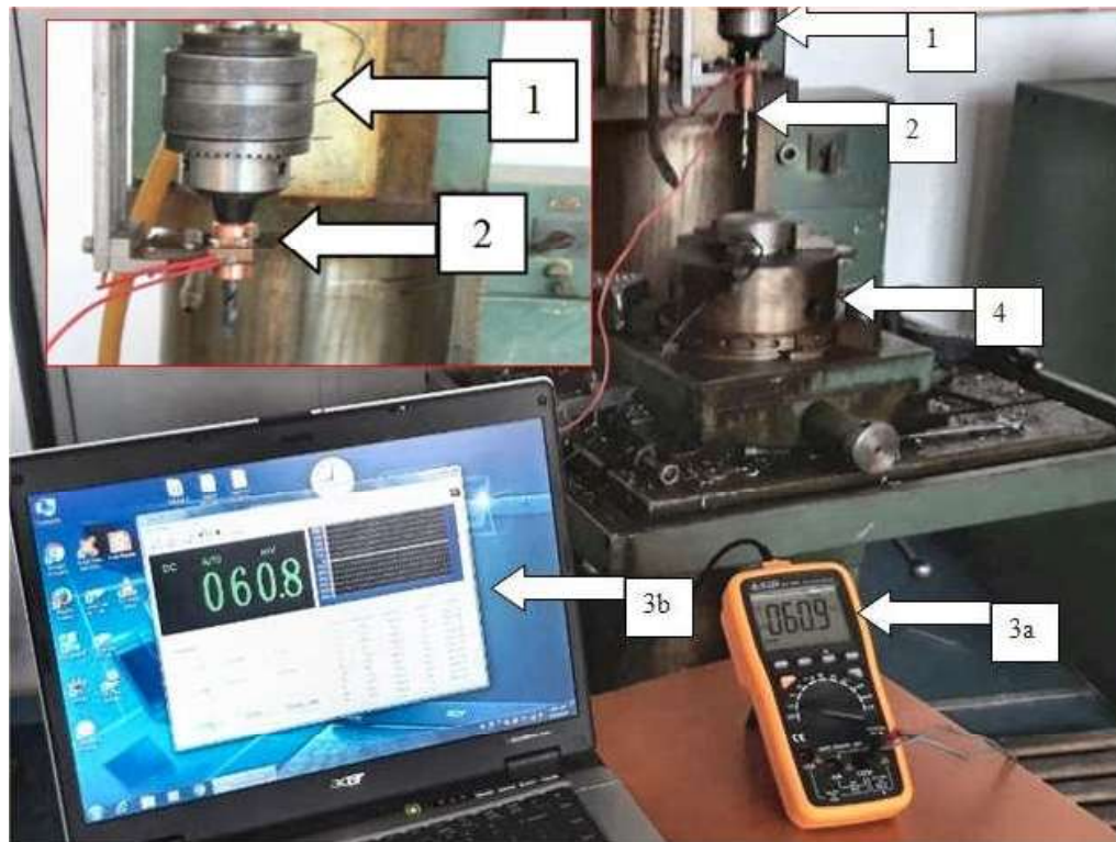
Figure 3. Experimental stand for measuring electrical current at drilling.
