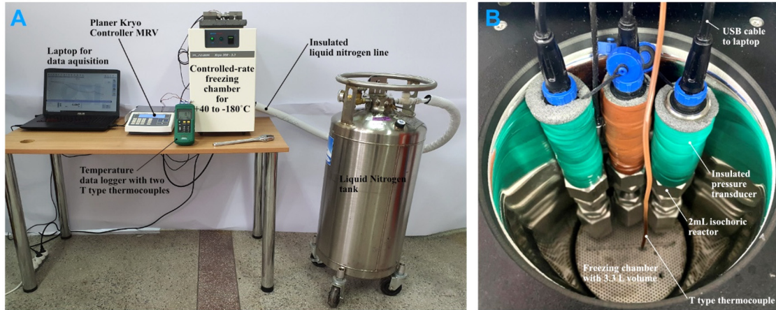
FIG. 2. (a) Photograph of the experimental system with the isochoric setup using the cryogenic freezer; (b) Photograph of the isochoric reactors inside the controlled-rate cryogenic freezing chamber.
