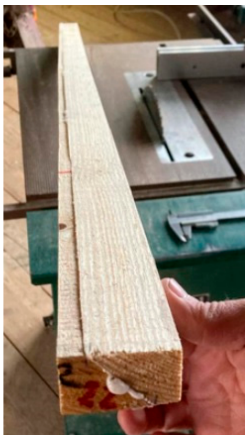
Figure 4. Reconstituted board after edge-cutting at 45^\circ , anti-parallel rotation at 180^\circ , and gluing of two tapered mirrored sideboards.
