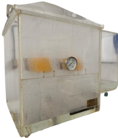
Fig. 1. Experimental setup for the salt spray chamber.
