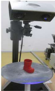
Figure 2. COMET L3D and scanning result. Figure 3. Default cloud of points. Figure 4. Patch surfaces
