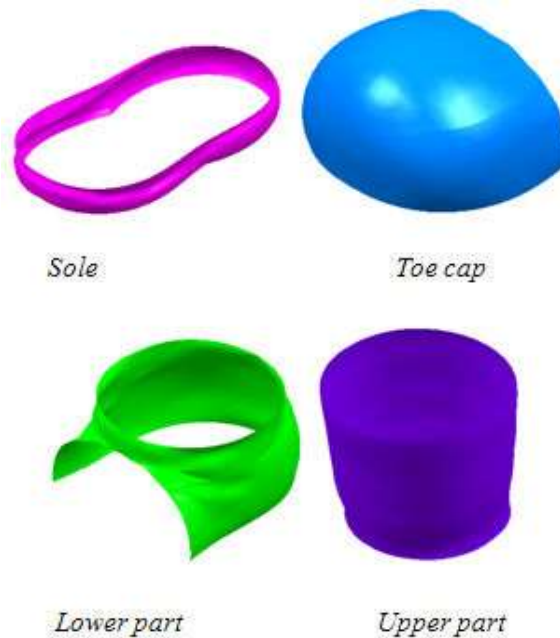
Figure 12. Boot components obtained using automatically generated curve networks
