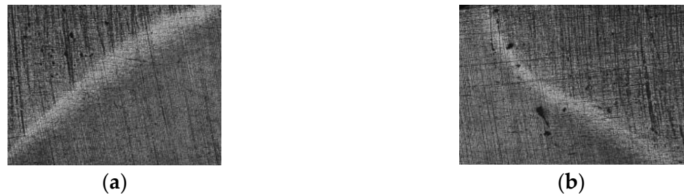
Figure 1. Macroscopic image of the test specimens welded: (a) without vibrations; (b) with vibrations; magnification: 10 \times .
