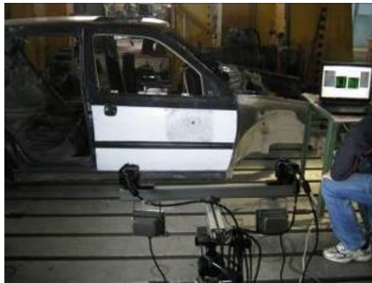
Figure 23. Door surface monitoring with VIC-3D system.
