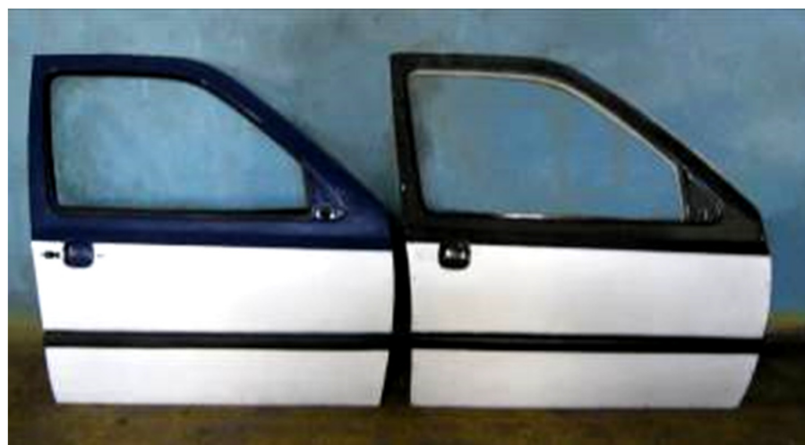
Figure 15. Metal door (left) and composite materials door (right).
