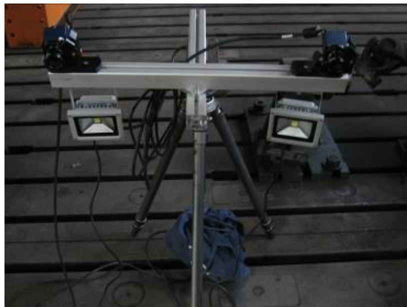
Figure 16. 1. High resolution video camera; 2. support; 3. tripod; 4. LED lamp. Basic elements of the VIC-3D system.
