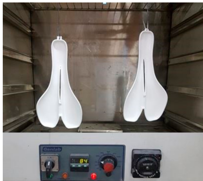
Figure 9. Heat treatment of the molds in the oven.
