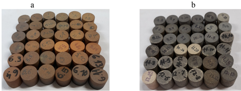
Fig. 1. (a) Composite with clay matrix reinforced Al 2 O 3 , SiC, Cu, Fe si Al particles; (b) Composite with bentonite matrix reinforced Al 2 O 3 , SiC, Al si Fe particles.
