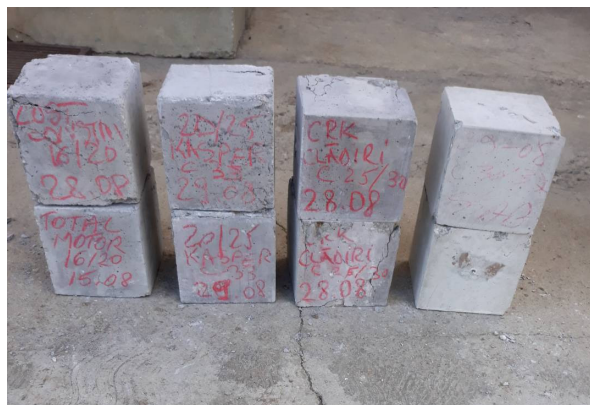
Figure 2. Compression-tested samples, waiting for optical microscopy.
