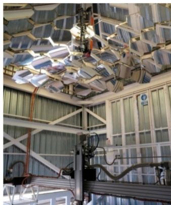
Figure 1. SF5 vertical axis solar furnace (test room).
