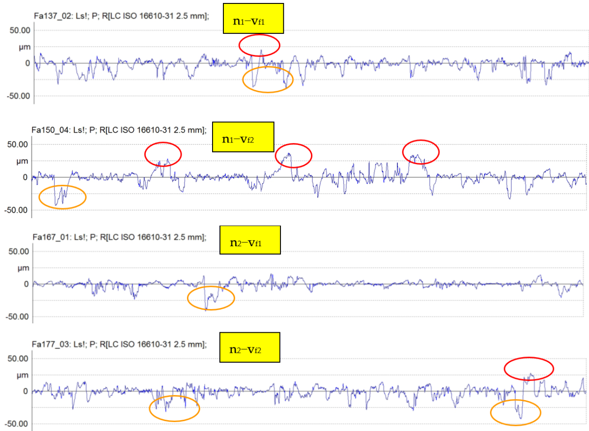
Figure 8. Roughness profiles of each group combination, rotation speed–feed speed. Raised fibers are marked with red; deep isolated valleys are marked with yellow ellipses.
