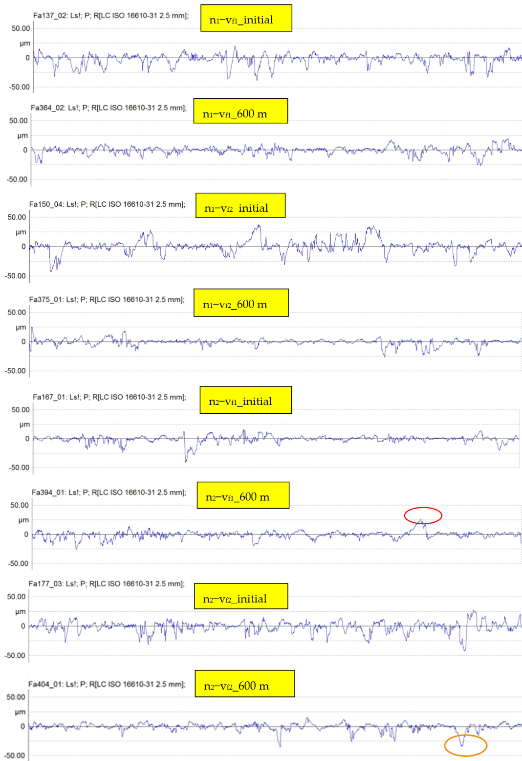
Figure 17. Roughness profiles of each group combination, rotation speed–feed speed comparing the effect of tool condition (when new and sharpened and after 600 m cutting distance). Raised fibers are marked with red; deep isolated valleys are marked with yellow ellipse.
