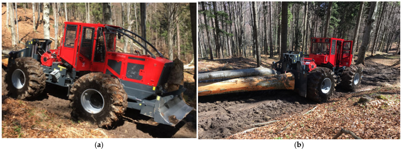
Figure 2. Description of the machine: (a) general overview on the TAF 2012 skidder; (b) TAF 2012 skidder during a loaded turn.
