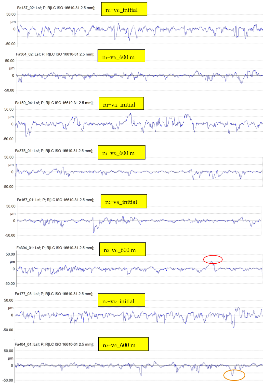
Figure 17. Roughness profiles of each group combination, rotation speed–feed speed comparing the effect of tool condition (when new and sharpened and after 600 m cutting distance). Raised fibers are marked with red; deep isolated valleys are marked with yellow ellipse.
