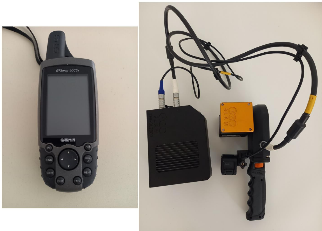
Figure A1. The two instruments used for measurements. Garmin GPSMap 60CSx (on the left) and GeoSLAM-Zeb-Revo (on the right).
