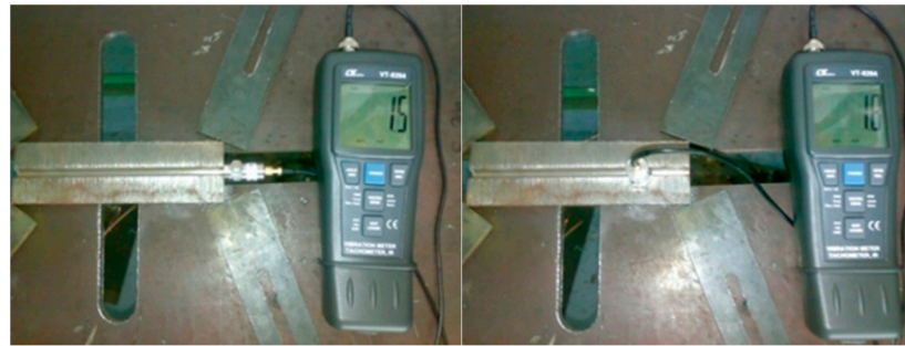
Figure 5. VAW acceleration measurement in the weld direction a_x , and in the perpendicular direction a_z .
