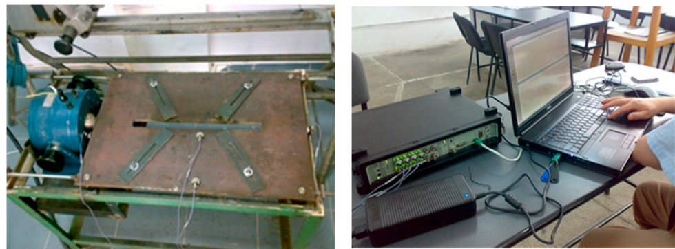
Figure 3. Dynamic signal analyzer pulse system—Type 3560 C-E01.
