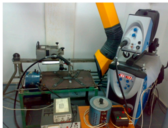
Figure 4. Equipment used for vibration-assisted welding.
