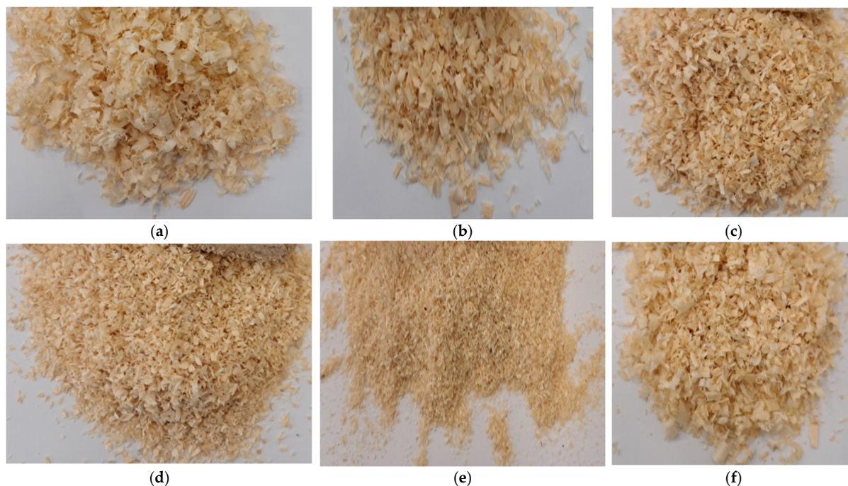
Figure 2. The sawdust used during the experiment (fractional composition of pine wood in the form of shavings): (a)-fraction greater than 4 mm; (b)-fraction of 3–4 mm; (c)-fraction of 2–3 mm; (d)-fraction of 1–2 mm; (e)-fraction less than 1 mm; (f)-unfracted sawdust (whole).
