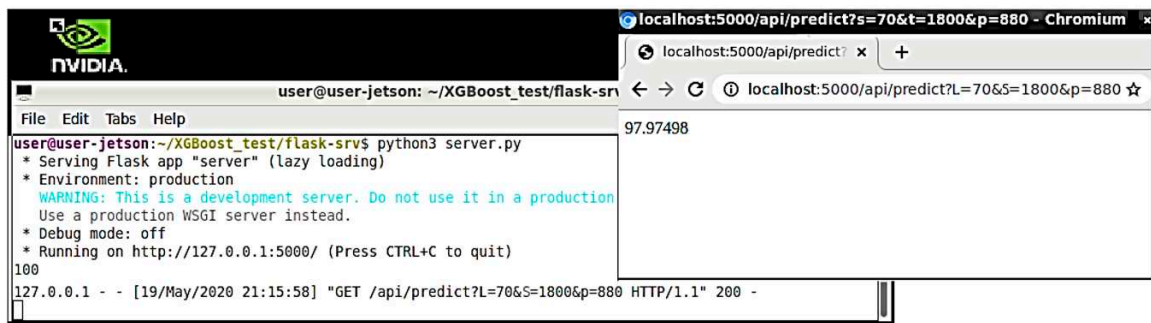
Figure 19. LXDE (light-weight X11) directives, intranet ANN invoking, and Pe prediction publishing using a normal browser.
