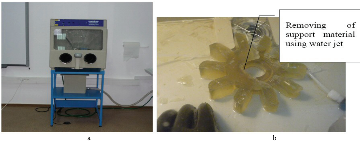
Fig. 10. a) Water jet recycle station, Transilvania University of Brasov; b) Pelton postprocessing method
