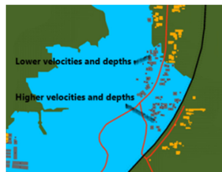
Figure 10. Location of flooded houses in Scenario 1 and distribution of low and high depths and velocities.
