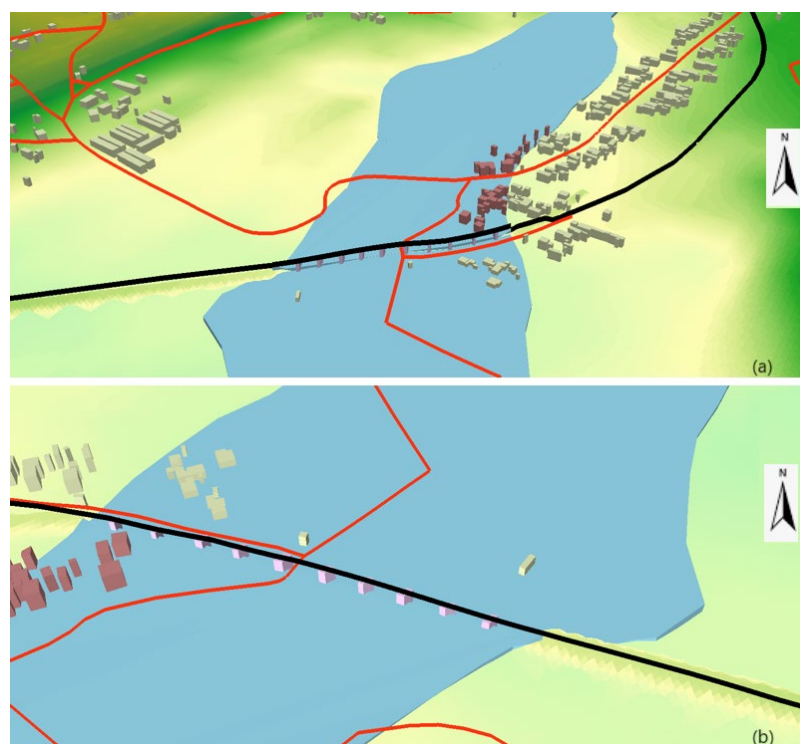
Figure 12. 3D representation of the hypothetical situation for a flood with an exceedance probability of 1%. (a) View from the south of the flooded surface, embankments, extended bridge, and affected buildings with red; (b) zoom in from the northwest on the 10-pillar bridge.
