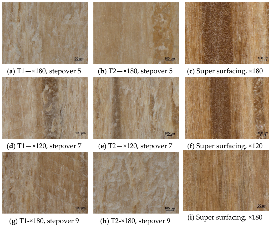
Figure 13. Comparative microscopic images of oak processed by T1 and T2 at the cutting depth of 1 mm and of the reference surface.
