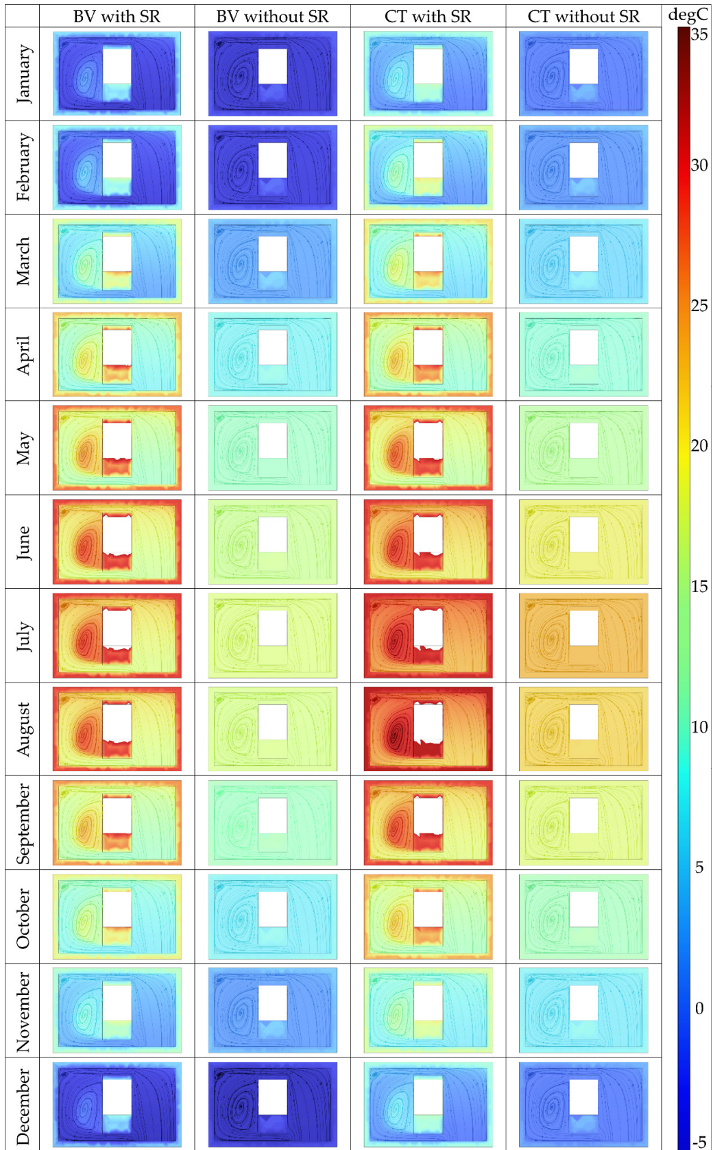
Figure 13. Cross-sections through air cavities for all four cases representing temperature variation.
