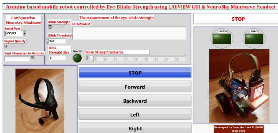
Figure 3 The graphical user interface of the LabVIEW application aimed to control the Arduino based mobile robot by using the voluntary eye-blinks
