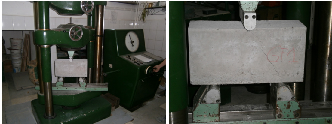
Fig. 6. GF1 beam between the press platforms (left.) and the moment of the first crack occurrence (right)
