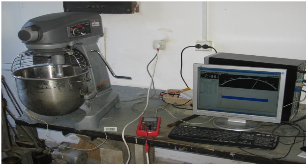
Figure 1. Workability measuring device.
