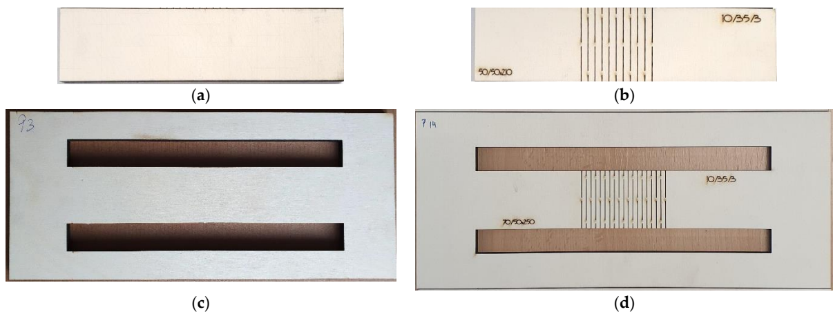
Figure 1. Four types of samples, tested in bending: (a) standard; (b) simple flexible; (c) framed rigid; (d) framed flexible.
