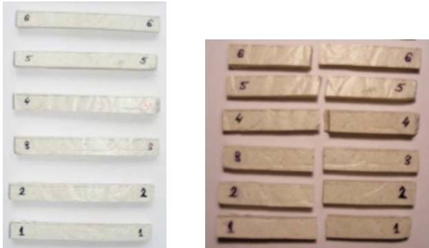
(a) Before bending test (b) After bending test Fig. 1. Specimens for bending test
