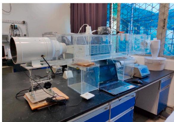
Fig. 27. Wind tunnel for dust removal characterization [76].
