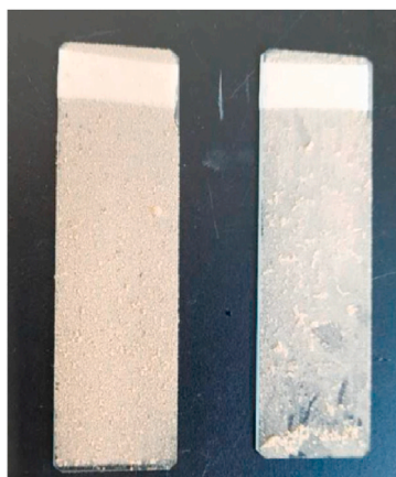
Fig. 36. Coated (right) and Uncoated (left) glass slides covered by A2 Test dust (ISO 12103-1) [70].
