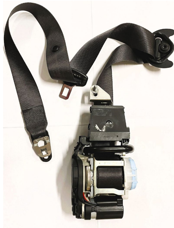
Figure 12. A 3-point seatbelt system with a pre-pretensioner and retractor mechanism.
