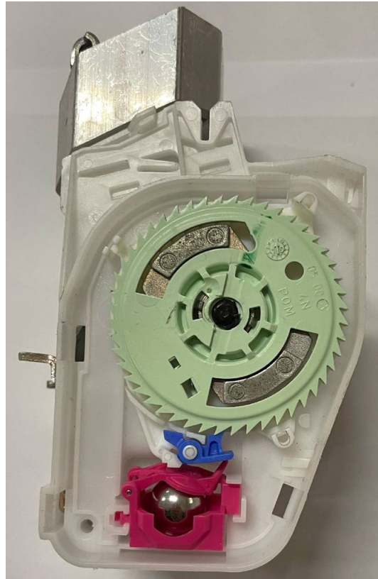
Figure 8. The ball-in-cup inertial locking mechanism.
