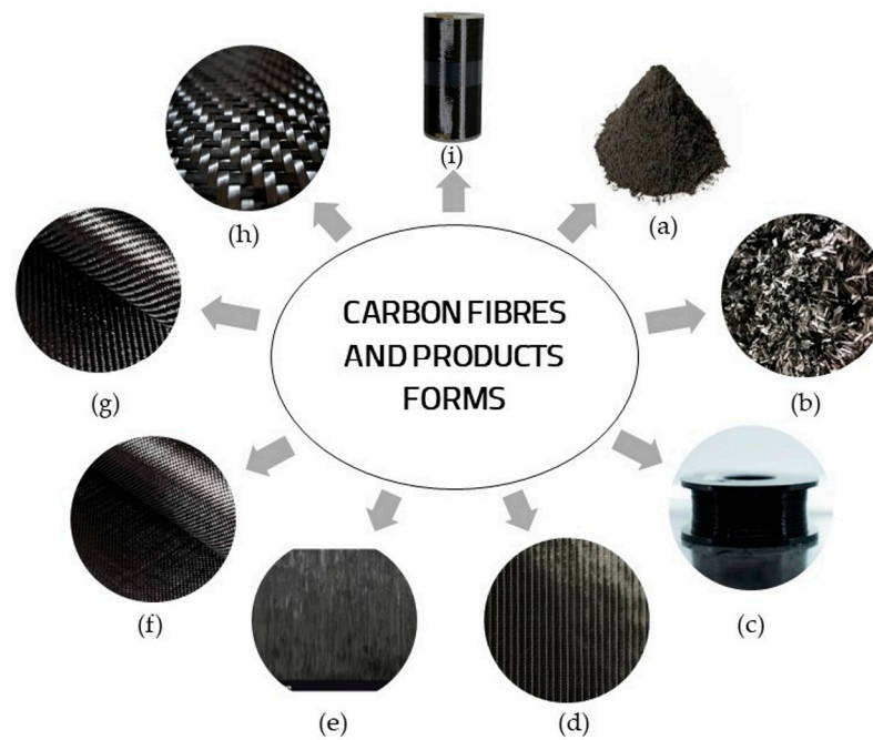
Figure 2. Carbon fibre and product forms: (a) milled fibres; (b) chopped fibres; (c) filament fibres; (d) biaxial fibres; (e) unidirectional fibres; (f) plain fabric; (g) twill fabric; (h) satin fabric and (i) unidirectional cloth.
