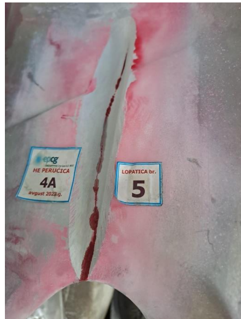
Figure 4. Groove on Pelton runner blade, on the back side.
