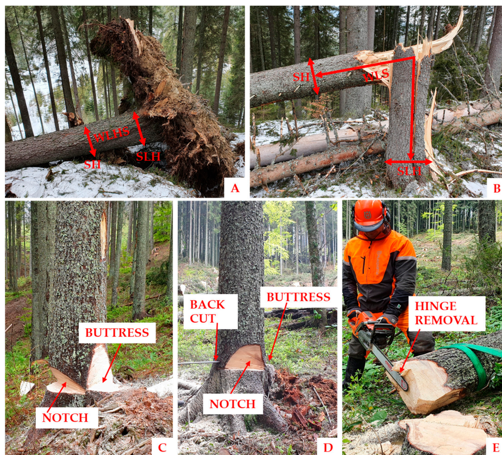
Figure 4. Wood losses: (A) WLHS—wood loss in high stumps; SH—stump height; SLH—stump legal height; (B) WLS—wood loss resulting from stem breaking and splitting; (C,D) wood loss because of the notch, buttress and back cut; (E) wood loss due to the removal of hinge wood.
